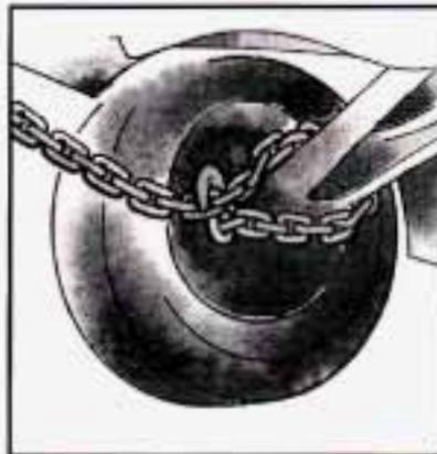
Attach a separate safety chain around the outboard end of both lateral arms.
