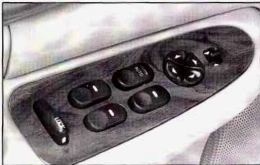
Switches on the driver's door armrest control each of the windows when the ignition is on. In addition, each passenger's door has a switch for its own window.
