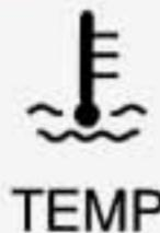
This light tells you that your engine coolant has overheated or your radiator cooling fan is not working.
