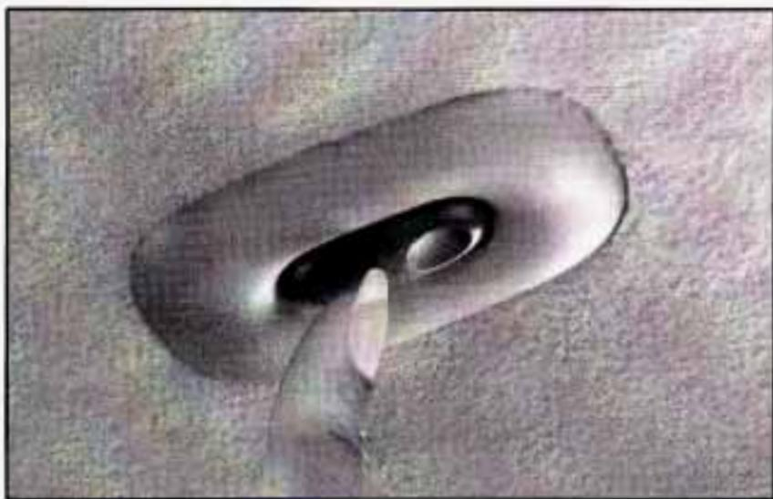
To open the sunroof, push the rear of the switch once and the sunroof will open to the vent position only. You will need to open the sunshade by hand.
