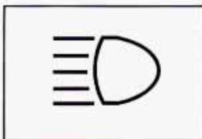
To change your headlamps from low beams to high beams, or high to low, pull the multifunction lever all the way toward you. Then release it.
