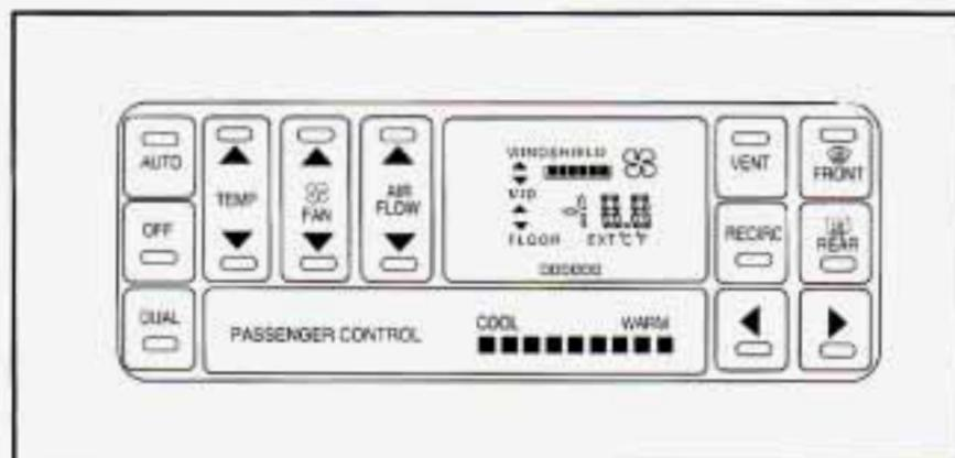
With this system, you set a temperature. You can then either let the system automatically control airflow direction and force to maintain the temperature, or you can manually adjust it. The system works best if you keep your windows closed while using it.
