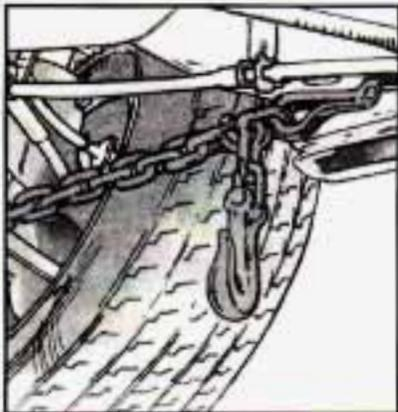
Attach T-hook chains into slots in the bottom of the floor pan, just ahead of the rear wheels, on both sides.
