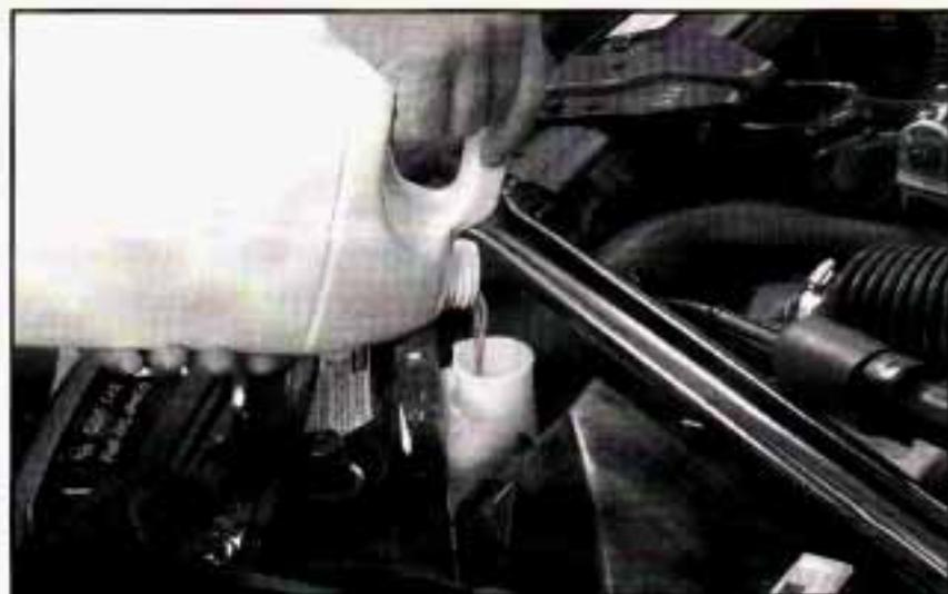
When the coolant in the coolant recovery tank is at the COLD mark, start your vehicle.
