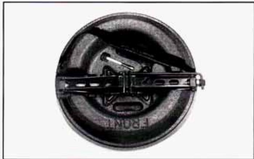
3. Turn the nut holding the jack to the left and remove it. Then remove the jack and wrench.
