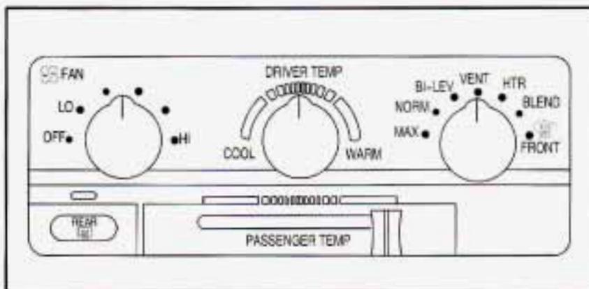
With this system, the driver and passenger can maintain separate temperatures. The system works best if you keep your windows closed while using it.
