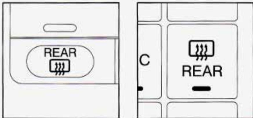
The rear window defogger uses a warming grid to remove fog from the rear window. Press the button to turn the rear defogger on. It will turn itself off after about 10 minutes. The picture above on the left refers to the defogger button that is found on a Manual Single Zone Climate Control System or Dual ComforTemp Climate Control System; the button on the right is found on the Dual Automatic ComforTemp System.
