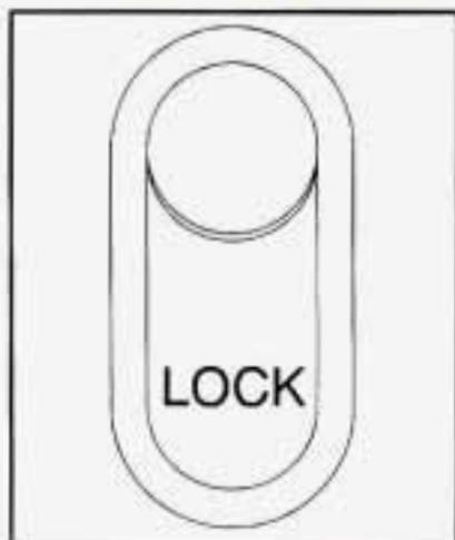
Press the power door lock switch to lock or unlock all doors.
