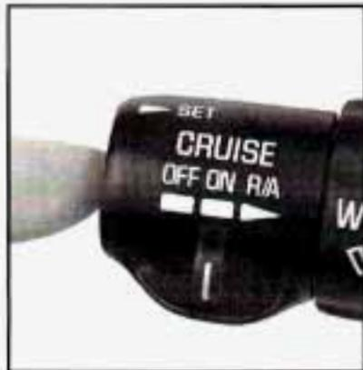
3. Push in the SET/COAST button at the end of the lever and release it. The CRUISE light on the instrument panel will come on.
