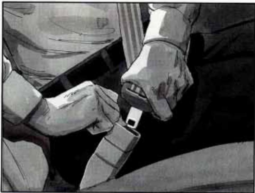
To unlash the belt, just push the button on the buckle. The belt should go back out of the way.
