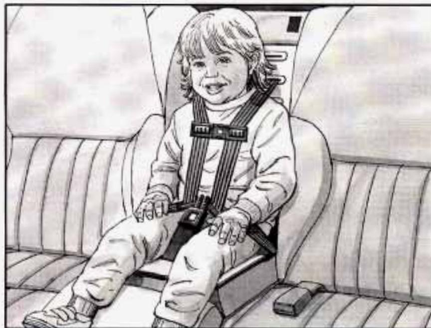
10. Adjust the position of the harness on the child's shoulders by moving the clip up or down along the harness. On each side of the harness, the shoulder part should be centered on the child's shoulder. The harness should be away from the child's face and neck, but not falling off the child's shoulders.
