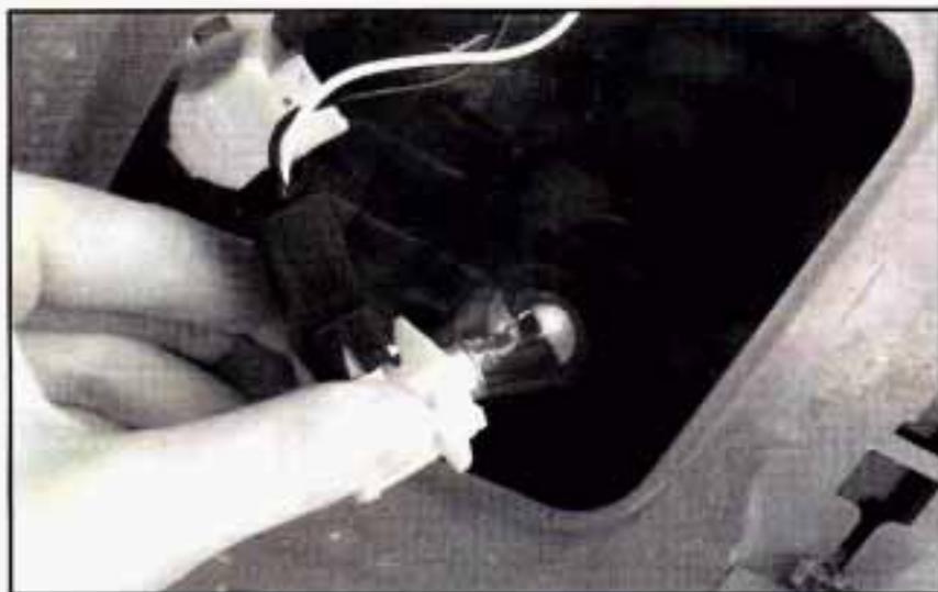
3. Remove the bulb by turning it one-quarter of a turn right to left.
