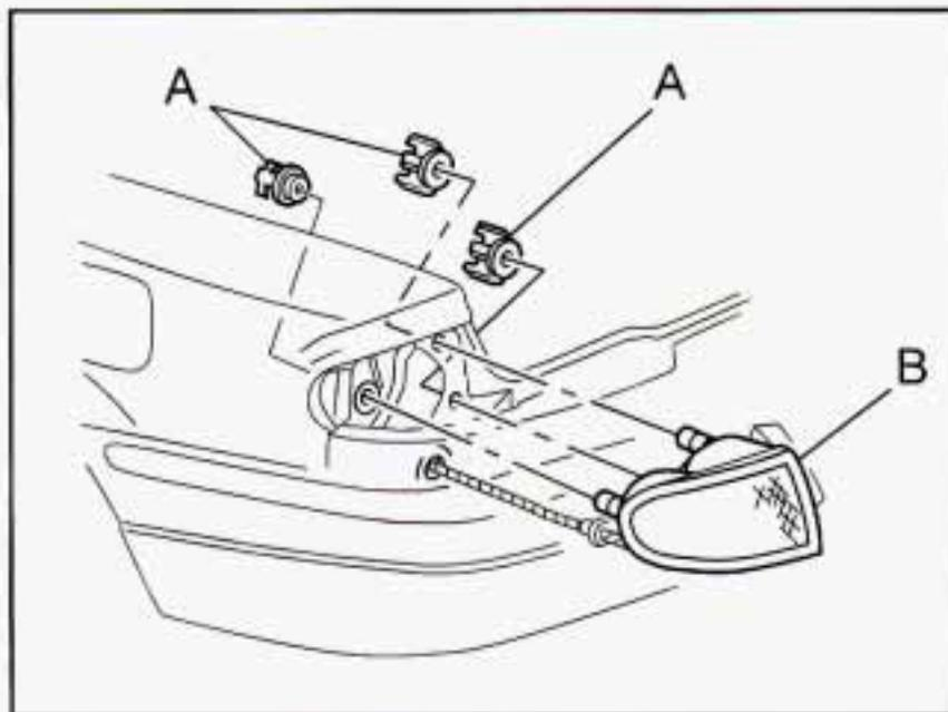
2. Pull the taillamp housing away from the body of the vehicle (B).
